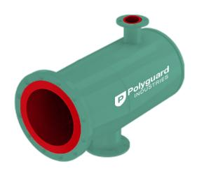
**Metal spools lined with special formulation Polyurethane to withstand the harshest wear applications.** Typically used for slurry transfer including mineral processing plants concentrate pipelines, tailings pipelines, oil sands pipelines. Also used for transfer of fluids containing abrasive solids at high pressure and high flow speeds where the Polyurethane liner is exposed to a highly corrosive environment.
